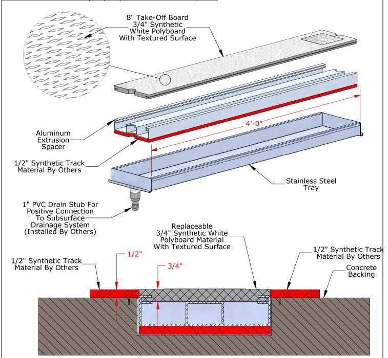
This Board should **ONLY** be used with proper track spikes at all levels of practice and/or competition. If track spikes are <u>NOT</u> used, the track surface side of the insert or blanking lid should be facing up.
